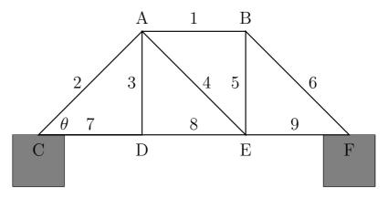
There are several external forces acting on the bridge, see below. There are loads (weight to be carried) at each of the joints,  $L_A-L_F$  that pull downward, and support loads from the left and right,  $S_L, S_R$  that hold the bridge up, and outward pressure P that pushes outward at the right support. (It is assumed that there is no pressure pushing output on the left support.)
