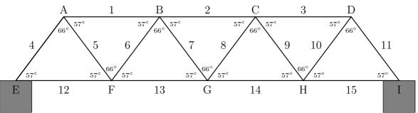
A two-axle truck drives across the bridge. It weighs 12,000 kg; with the weight evenly divided between its axles. The axles are 5 m apart.
