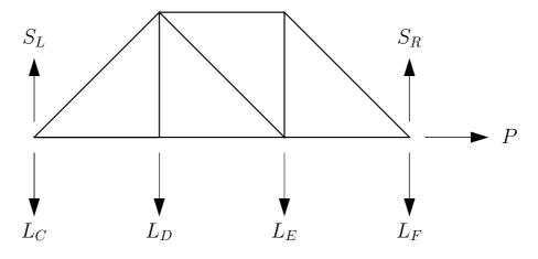
The forces internal to the bridge are compression/tension on the bridge elements,  $f_1, \ldots, f_9$ . These act along the beams with a positive sign representing tension and negative representing compression. In this model there is no torsion or twisting at the joints; however, in the real world there may be.
