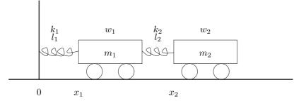
The length of the first spring is  $x_1$  so the outward force it exerts is equal to  $F_1 = k_1(l_1 - x_1)$ . The second spring's length is  $x_2 - x_1 - w_1$ , so exerts an outward force of  $k_2(l_2 - x_2 + x_2 + w_1)$ .
